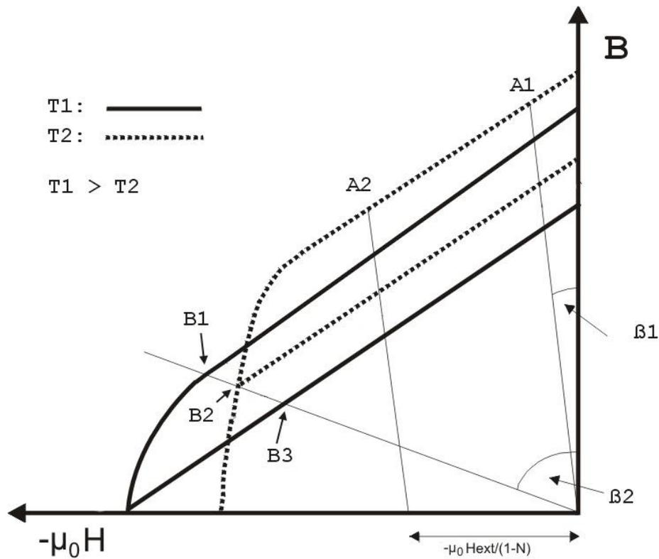
**Fig. C1:** Demagnetization curves with working points and load lines under different temperatures and external fields.
